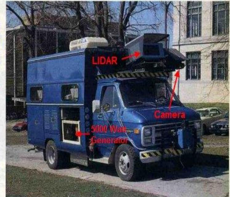
Photo 1: The NAVLAB autonomous navigation test-bed vehicle and the road used for trial runs.
