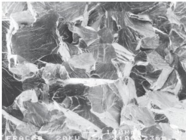
Figura 30: Fratura intergranular que caracteriza o defeito rock candy . Fonte: Metal Failures: Mechanisms, Analysis, Prevention, Second Edition. Arthur J. McEvily (2013)
