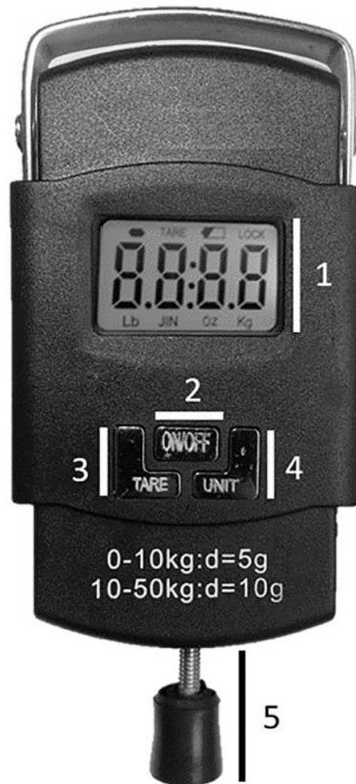
Figure 1 Adapted pressure algometer—PA. (1) Display; (2) On-Off button; (3) Tare button; (4) Unit selection button; (5) Adapted terminal.
