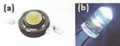
Figura 3: Dois tipos de LEDs brancos: (a) LED HP e (b) LED HB
