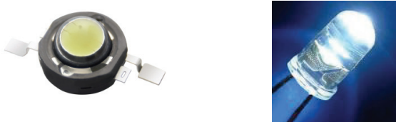
Fig. 2. HP (left) and HB (right) LED types.
