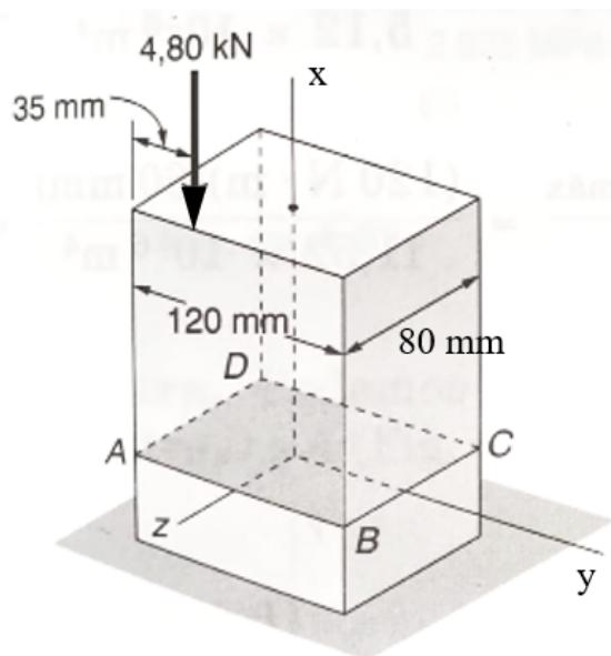
**Respostas:**  $\sigma_A = -2,625 \text{ MPa}$ ,  $\sigma_B = -1,375 \text{ MPa}$ ,  $\sigma_C = 1,625 \text{ MPa}$ ,  $\sigma_D = 0,375 \text{ MPa}$
