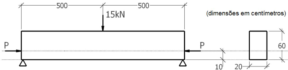
**Respostas:**  $P_{\max} = 80 \text{ kN}$ ;  $\sigma_{\max}^T = 1,125 \text{ MPa}$ ;  $\sigma_{\max}^C = -2,458 \text{ MPa}$
