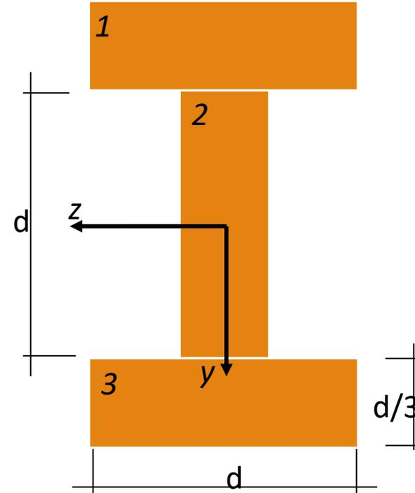
$$I_y = \frac{h_1 b_1^3}{12} + \frac{h_2 b_2^3}{12} + \frac{h_3 b_3^3}{12} = \frac{(d/3)d^3}{12} + \frac{d(d/3)^3}{12} + \frac{(d/3)d^3}{12}$$
