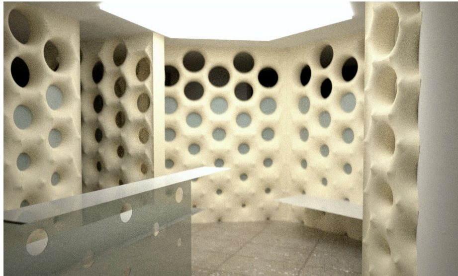
Figure 11: Alberto T. Estévez, Consulting room , Barcelona, 2008-09: panels manufactured using the CNC milling machine of the Digital Architecture Laboratory of the Research Group.
