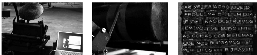
FIGURE 6 – Images of typesetting and sensor coupled to the press and to the computer to print movies. Source: Claudio Santos acquis.
